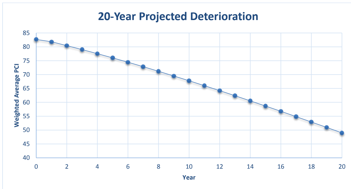
Figure III.A: The projected deterioration developed for the bituminous pavements in the City of Rogers over the next 20 years since 2018 inspection.
